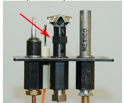
9. Using a 7/16" wrench turn the nut counterclockwise until the pilot starts to turn.
