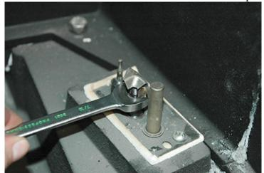
10. Continue to unscrew the pilot from the assembly until you can lift the pilot out.
