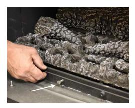
5. Very carefully remove the log set. It is very fragile and should be supported with two hands under the base. If the base of the log set is damaged the log set should be replaced.
